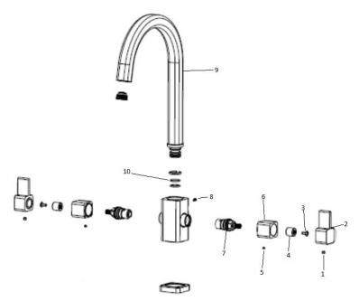
retaining screw (5) with a 2.5mm allen key and then unscrew the valve cover (6). You will then be able to remove the valve (7) by using an adjustable spanner and fit the replacement parts.
